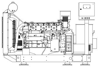
Dimensions L x W x  $H_1/H_2$  (mm), not for installation D7A T / UCM274D-1 2410 x 1157 x 1275/1631
